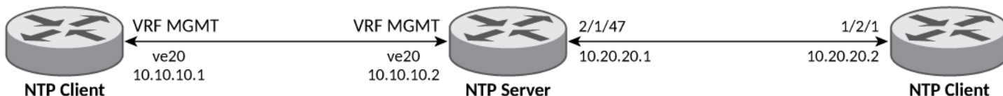
FIGURE 4 Use Case 2: NTP Server over Management VRF with One Client Using Management VRF and Another Client Using Ethernet
