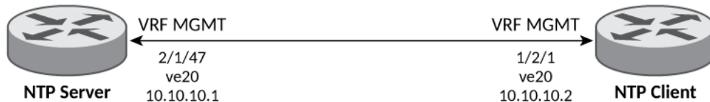
FIGURE 3 Use Case 1: Management VRF Forwarding with One Client and One Server on VE
